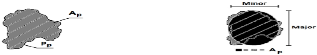
Fig. 5: Schematic of shape factors [19]; A_p = Area of particle, P_p = Perimeter of particle
